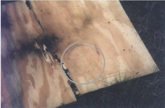
Imprint (with readable nomenclature) of the jar's end cap in the test box walls. Note, oddly, that the cap struck somewhat off-center from the main force of the explosion. This indicates that the jar did not disintegrate uniformly.
